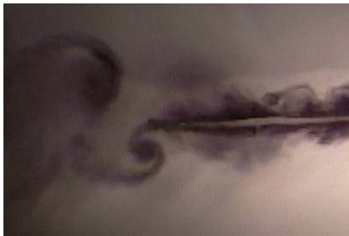
Figure 4. Dye visualization of near wake of the flapping flexible membrane. Flow is from right to left. Aspect ratio s/c=0.22 , St \cong 0.6 .
